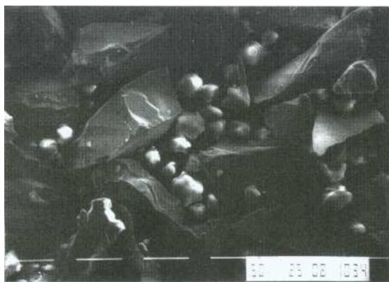
Fig. 26-7. SEM of air abrasion particles* composed of a mixture of 50 gm alumina (dark irregular particles) and smaller silicate particles (light color) used for final abrasion of metals during which a molecular coating of silicate is tribochemically deposited on the metal. This silicate layer on the metal allows reaction with a silane-priming solution for subsequent bonding of resin to the metal.
