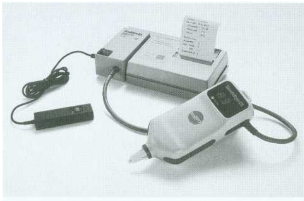
Fig. 23-10. ShadeEye-EX Chroma Meter. This device uses a colorimeter to measure tooth color and processes the information into formulae for fabricating a metal-ceramic restoration. (Courtesy Shofu, Inc.)
