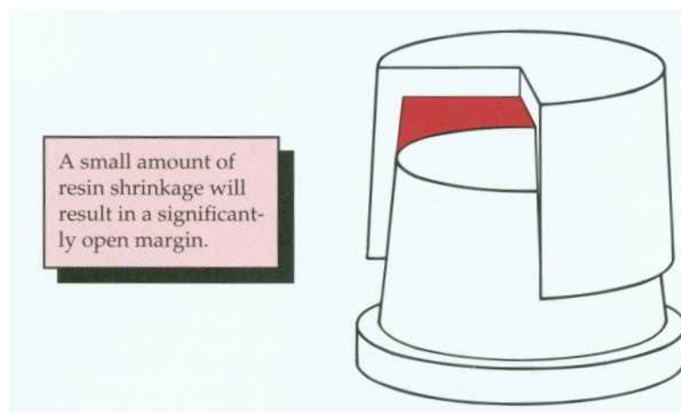
Fig. 15-24. With ideal axial wall convergence, a 2% reduction in crown diameter results in a comparatively high marginal discrepancy.
