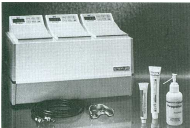
Fig. 14-23. Hydrocolloid conditioning equipment consists of three thermostatically controlled water baths: boiling, storage, and tempering. (Courtesy Van R Dental Products, Inc.)
