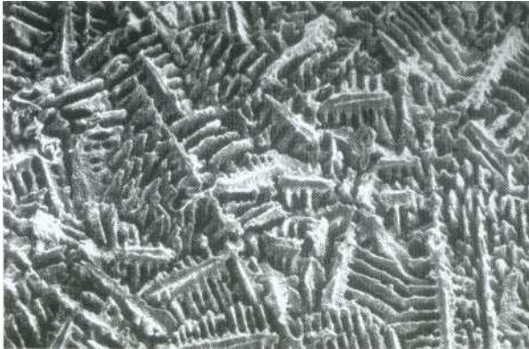
Fig. 26-3. Scanning electron micrograph (SEM) at 1000x magnification of a Ni-Cr-Mo-Al-Be alloy electrolytically etched. The microstructure is selectively removed to create a highly undercut surface that can be wet by hydrophobic composite resins.
