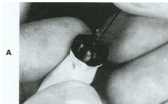
Fig. 22-10. Spruing technique for a single casting. A, Attaching the sprue to the pattern. B, Removing the pattern from the die.
