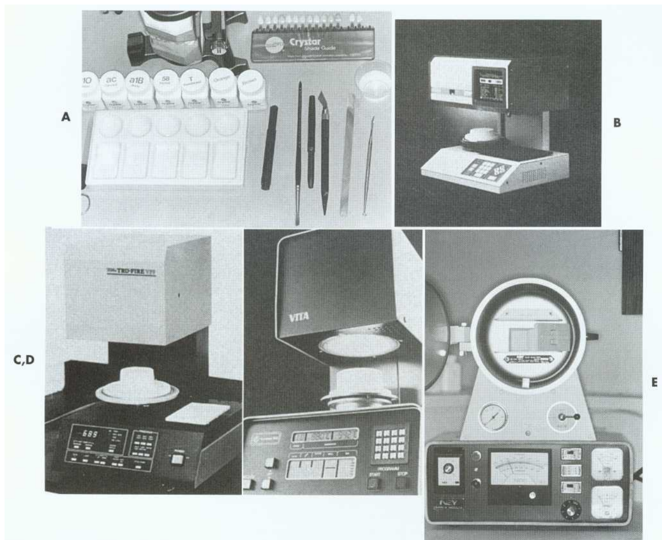
Fig. 24-20. A, Armamentarium for porcelain application. B, CMP KC 2000. Vacuum porcelain furnaces C, Jelenko Tru-Fire VPF; D, Vita Vacumat; E, Ney Mark 111. (B courtesy CMP Industries, Inc. D courtesy Vident.)
