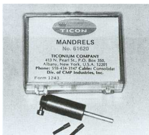
Fig. 28-11. Ticon mandrels are prefabricated inserts embedded in the wax pattern. The retainer is cast directly onto the mandrel to form the female component of the connector.
